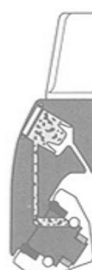
Sealed friction bearing (IADC xx6 or xx7)
